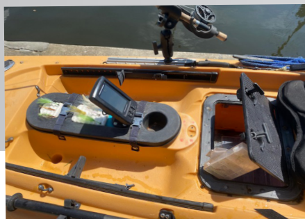
A fish finder and live well come in handy. Live well uses battery-powered aerator.
