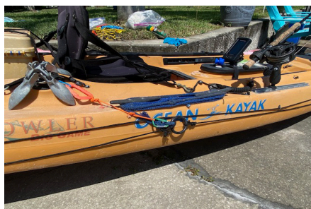
An anchor trolley lets you control which way your kayak faces. For example, if you are anchored in current, such as a changing tide, and you are facing away from where you are fishing, the anchor trolley will turn you around by moving the anchor rope to the opposite end of the kayak.
